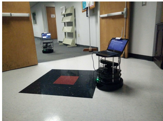
Fig. 1: The robots, TurtleBots 2 equipped with a WiFi dongle, deployed in an environment to build its communication map.
